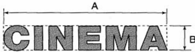
Figure 4 MEASURING SIGN AREA
