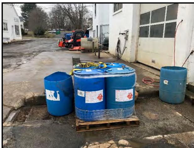
Figure 4-31: Outside storage of liquid materials without an overhead cover or secondary containment at HSI10.
