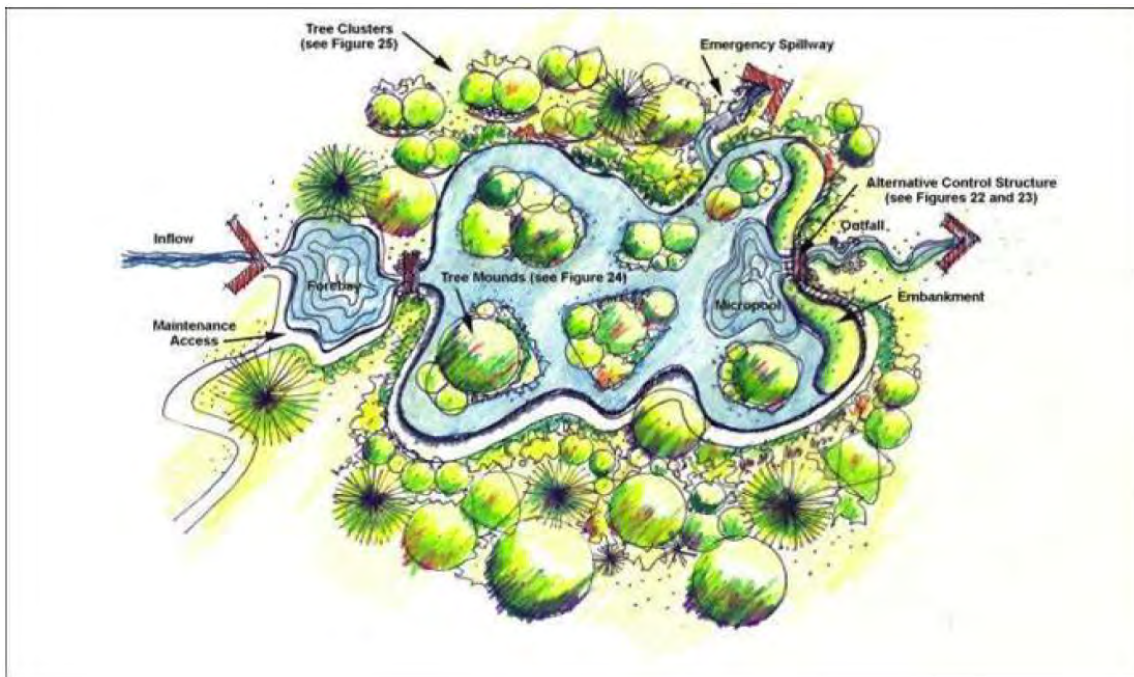
Figure 5-1: Constructed Wetland Standard Concept Design (Virginia DEQ 2011a)
