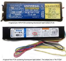
A typical Non-PCB containing fluorescent light ballast. The ballast has a "No PCBs" marking on the top of the ballast and the text "electronic ballast". Only magnetic fluore light ballasts contained PCRs
