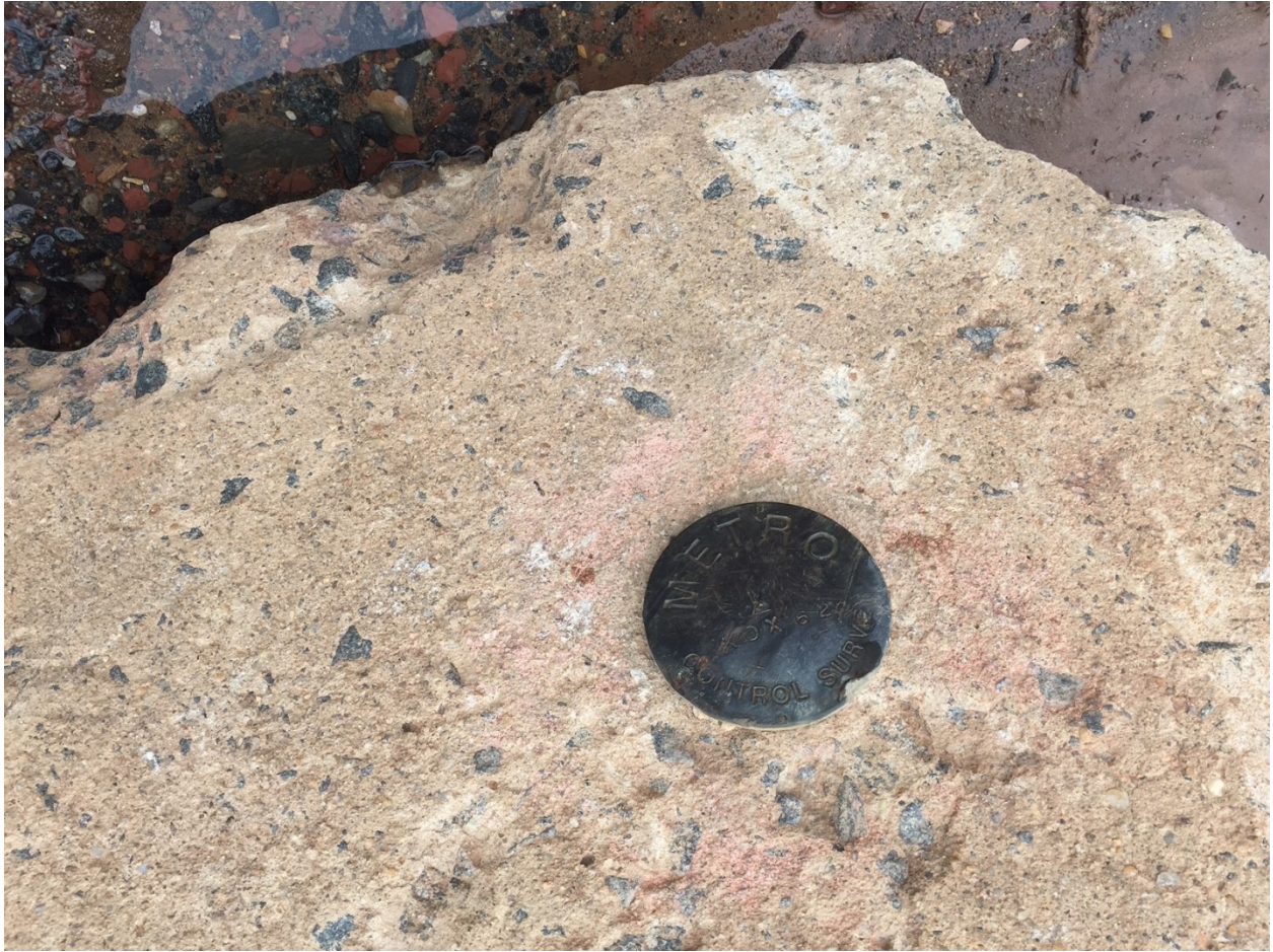
Photo 2. Survey marker on a large block of concrete. Marker suggests that this block originated from a Metro Project.
