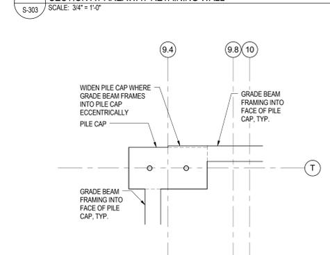
4 GRADE BEAM FRAMING ECCENTRICALLY INTO PILE CAP
