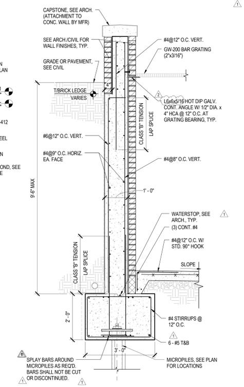
3 SECTION AT AREAWAY RETAINING WALL
