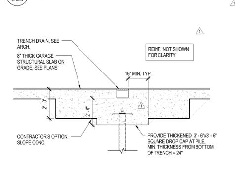
10 SECTION THRU THICKENED SLAB AT PILE
