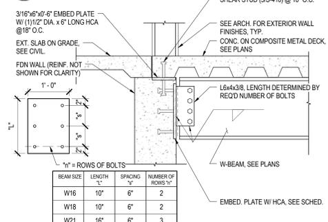
8 SHEAR CONNECTION AT CONC. FDN WALL (EMBED PLATE)
