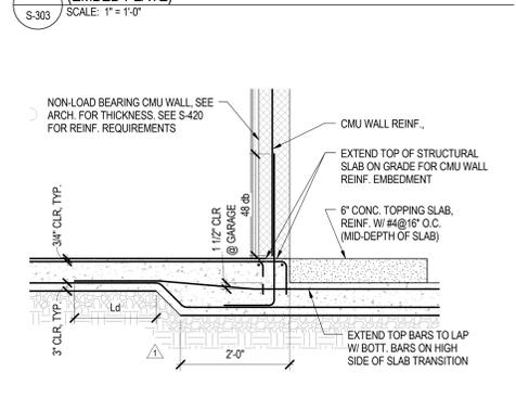
9 SECTION THROUGH STRUCTURAL SLAB ON GRADE STEP
