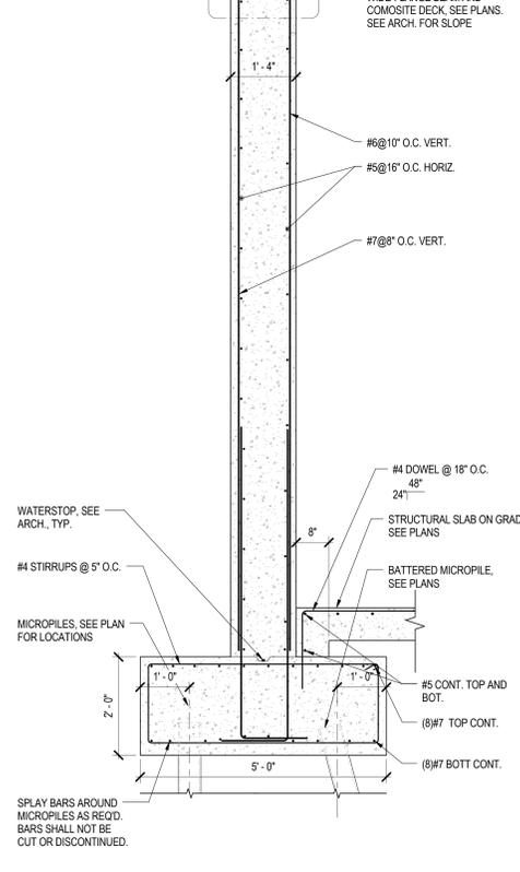
25 SECTION THRU BASEMENT WALL AT STAIR 1
