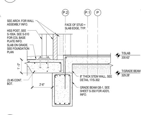
12 SECTION THRU GRADE BEAM @ MECHANICAL YARD
