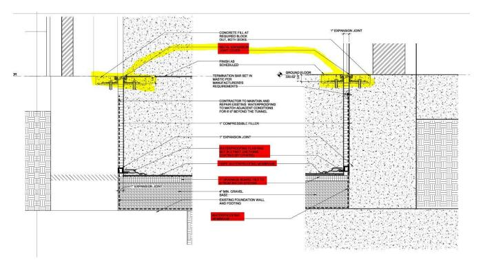
A33: The expansion joint for the tunnel is as specified in section 079300. Contractor shall disregard the "Metal Expansion Joint Cover" note indicated on the drawings.
