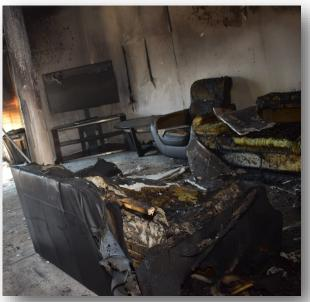
This fire was a result of a failure of lithium batteries in a laptop. It caused \$111,947 in damages.
