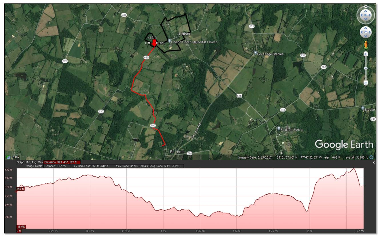
Figure 4-9 – Elevation Profile for Conceptual Layout Directly to St. Louis WWTP
