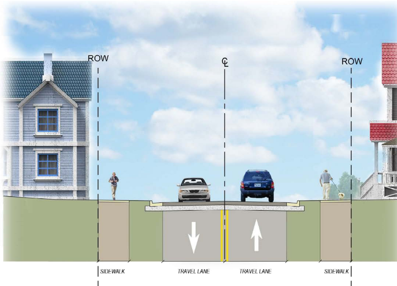
US Route 15: 2-Lane Undivided Curb and Gutter Typical Section
