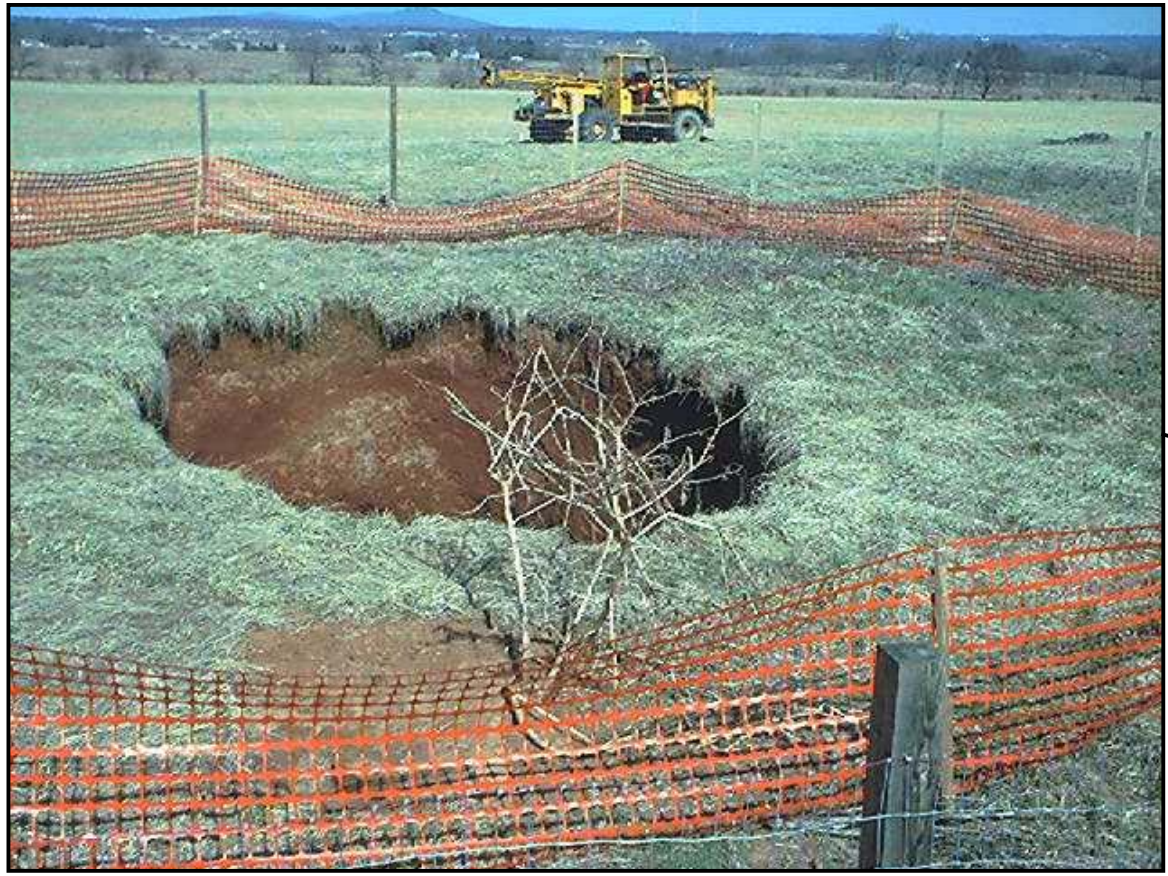
Selma Estates Subdivision (photograph date: March 27, 2003) The sinkhole is approximately 30 feet in diameter and 30 feet in depth and opened approximately 100 feet from a well being installed.
